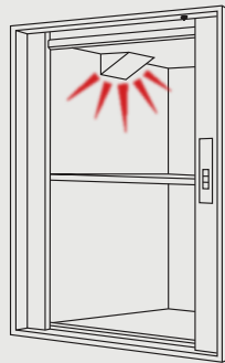
An infra-red car heater, positioned on lift car ceiling to heat the top shelf.
